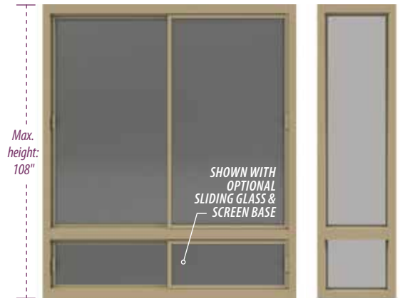
W2B Sliding glass window and base Overall window panel heights including base up to 108" Base height with fixed glass or aluminum 12" to 36" Base height with sliding glass 14" to 36"
